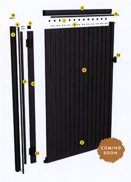
When calculating even spacing between vertical slats, overall gate width should be carefully considered to ensure first and last gap (between gate side frames and first/last slat) are kept uniform with other slat spacing
