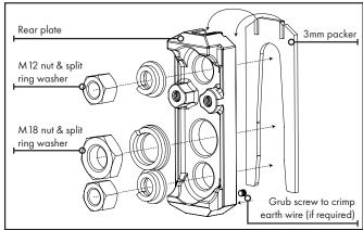
Secure the rear plate to substrate. Ensure rear plate installed with word 'TOP'
