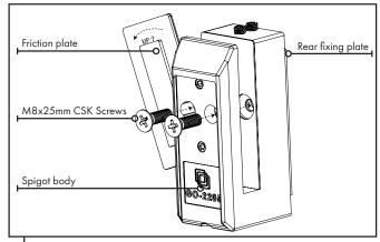
Remove friction plate from spigot body. Insert 2x M8x25mm counter sunk screws through holes in front and into back holes locating into threaded bosses in rear plate.
