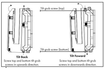
Before installing glass, use a spirit level to adjust spigot to vertical position. Recommended to use a string line from first to last spigot in alignment to ensure
