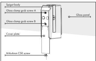
Install 12mm thick glass into spigot and tighten glass clamp grub screws A and B. Install cover plate by sliding upwards into recess at front of spigot.
