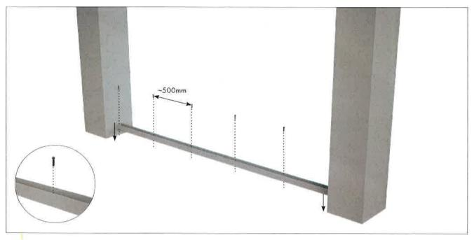
Install bottom U Channel to floor substrate at 500mm centres.
