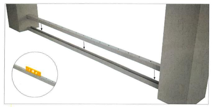
Insert the Horizontal Rail into bottom U Channel with machined holes visible (i.e. facing upwards), placing on U Shaped packers.
