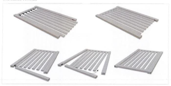
5 Insert palings into bottom rail. NOTE: Palings have a notch on one end - use notched end as BOTTOM of paling. When a Midrail is being used, spread both side frames and install the Top Rail into palings one-by-one. Once palings are installed into the Top Rail, slide both side frames into position, engaging the Midrail and Top Rail.
