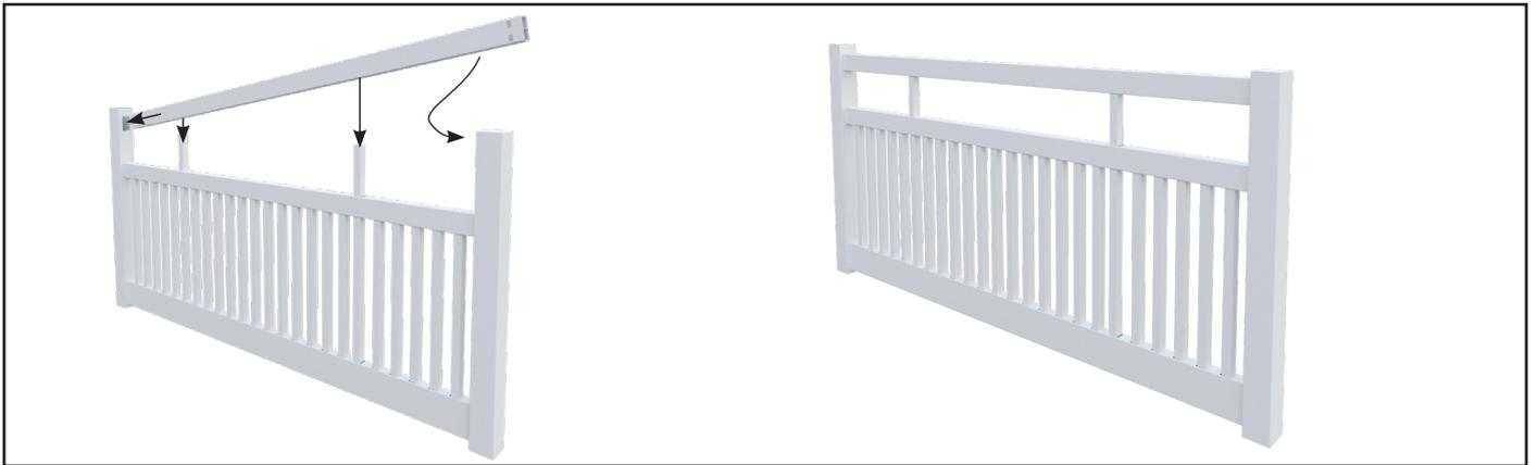
**12** Install top rail over long pickets guiding pickets into holes on underside of top rail. Insert top rail into one post and then lever into adjacent post.
