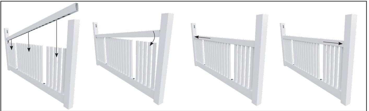
10 Push mid rail into slot on 1 post then lever into slot on adjacent post. Insert pickets as the mid-rail is levering down. Posts may flex to allow for insertion.
