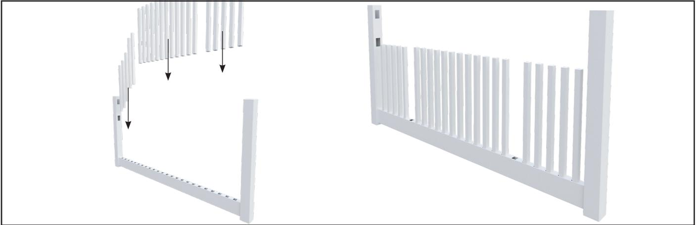
9 Install short pickets into bottom-rail leaving long pickets for subsequent step. The long pickets are positioned 6 pickets in from either end.
