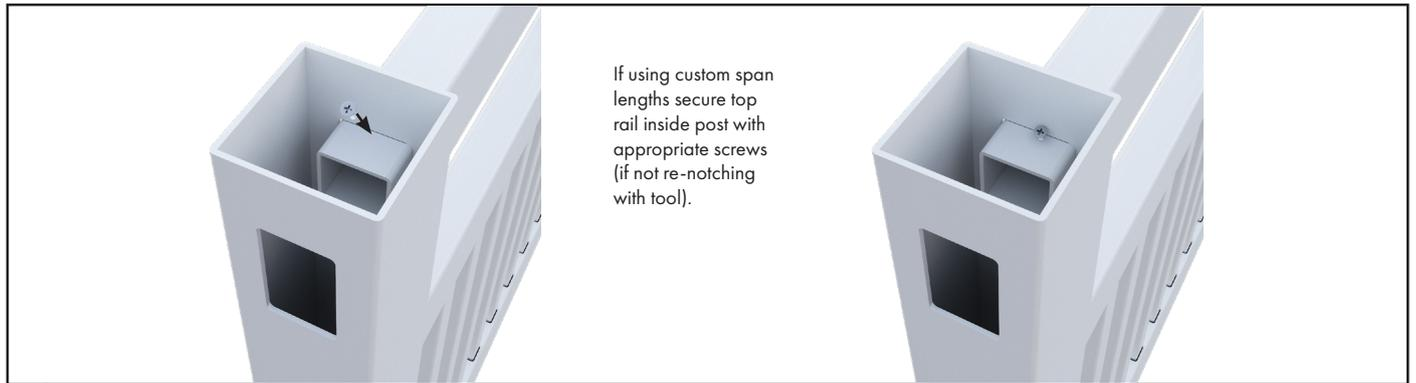
**\*\*** If using custom lengths, re-notch the tongues with notching tool (sold separately) or secure top rail in place on post using appropriate screws.
