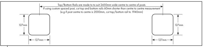
Top and bottom rails are supplied suited to 2450mm centre to centre post spacing.
