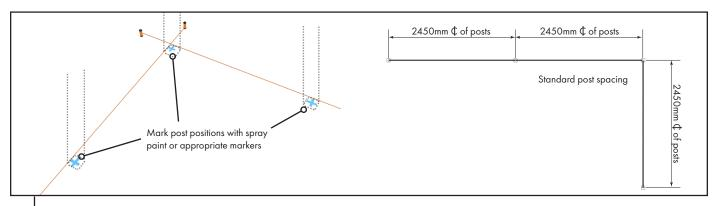
3 Mark post to post centres using appropriate markings such as spray paint or stakes. Standard fence panel post centres are at 2450mm. If using shorter spans, space posts appropriately.
