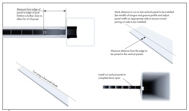
The last vertical panel in the span may need cutting to fit. Mark distance to cut on last vertical panel to be installed (be mindful of tongue and groove profile and adjust panel width on appropriate side to ensure correct joining on side to be installed) and cut using a fine tooth blade. Follow manufacturer's instructions for safe use of saw.
