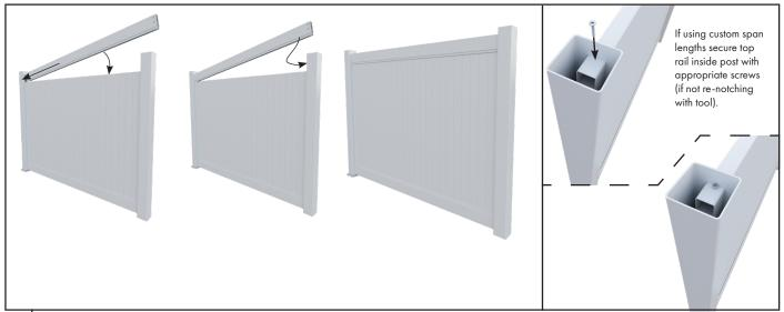
Install top rail over vertical panels and simultaneously push top rail as far as possible into one post and then slide back into adjacent post. Standard length top rails are self securing using the pre-notched tongues.
