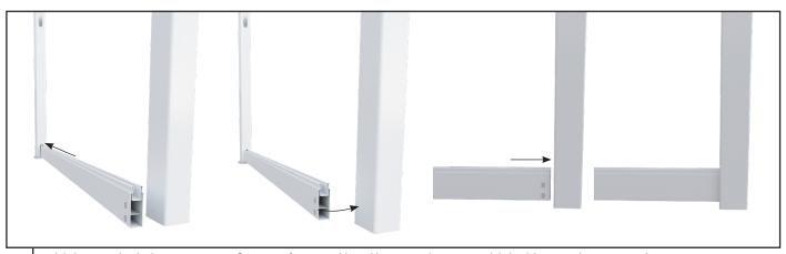
Slide bottom rail with aluminium insert into first post as far as possible and lever into adjacent post. Slide back bottom rail to ensure notches have passed into adjacent post.
