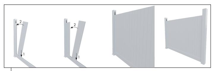
Starting at the vertical U channel on one side, insert vertical panels into bottom rail and lever into position. Repeat process towards the next post.
