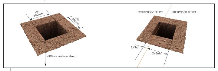
For in-ground installation dig holes for posts minimum 600mm deep by 300x300mm wide.
