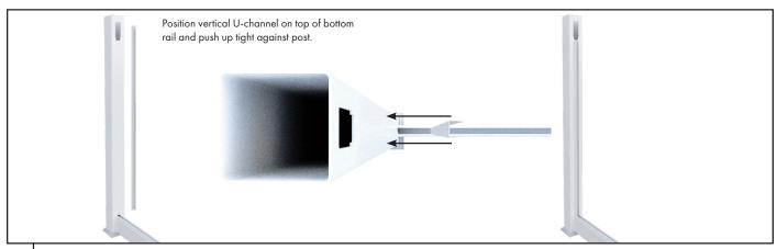
Position vertical U-channel on top of bottom rail and push up tight against post. Repeat step on all posts, where fence panels are to be installed. U channel will be held against post both sides once vertical panels installed (no fixing required).
