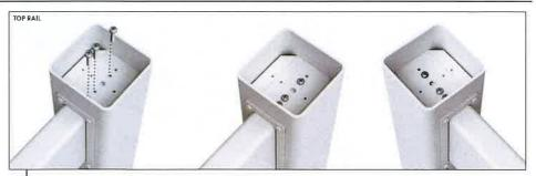
Screw top rail into place inside side frame using 3 x 25mm screws, Top plate is supplied fixed in position in side frame with holes pre-drilled for fixing through. Repeat on other side.
