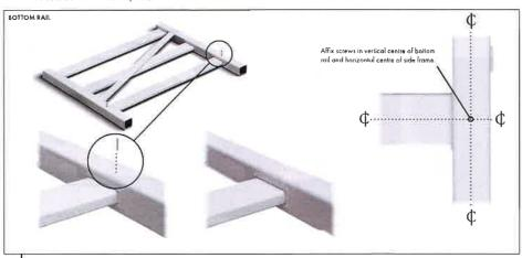
Ensure gate square. TIP - measure diagonals ensuring the same measurement. Screw fix off bottom rail through gate side frames using 1 x 50mm screw each side. Affix both sides at midpoint of bottom rail height and centre of post.
