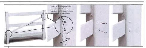
The cross member must be fixed off at hoth ends, Drill 2,5mm pilot holes 8mm in from edge of gate side frame. Fix off at bottom and top side of cross member using 2 x 50mm screws,
