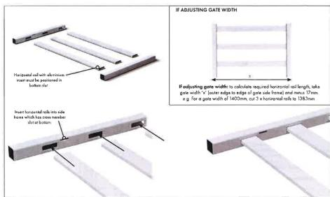
b Lay out side frames and horizontal rails on α flat bench.
