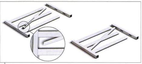
lnsert cross member into the gate side frame at bottom side (same side frame that horizontal rails have already been inserted).
