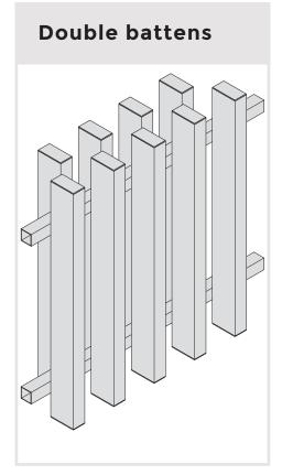
Battens come standard with 2x aluminium caps per batten (top and bottom) 45x45mm horizontal rail comes with 2x fixing brackets as standard
